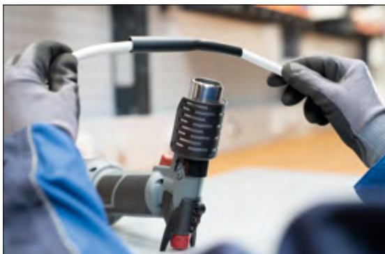
Applying heat shrink tubing hands-free.
