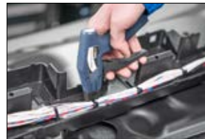
Secure cutting of cable tie straps with the EVO cut zip tie cutter.
