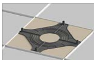
1. Place the SpotClip-Plate in position.
