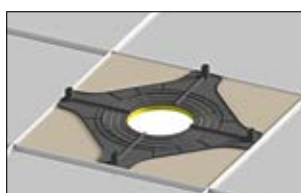
2. Cut the ceiling plate.
