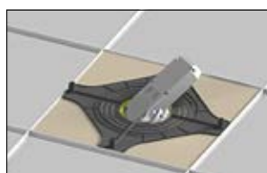
3. Insert the downlight through the cut hole.
