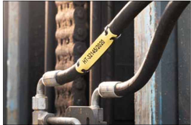
Cable marker for easy marking in tough environments.
