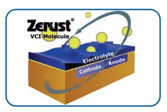
How the ZERUST® protective molecules suppress corrosion:
