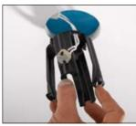
1. Squeeze the mounting legs to install SpotClip in the fixing hole.
