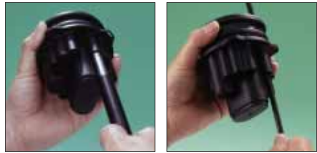
(1) Punch out base hole with port tool (2) Feed through cable
