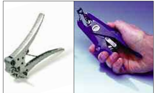
Sleeve expansion applicator tools ensures easy application of elastomeric products NA 8/10 (left), D, SS, S, K (right).
